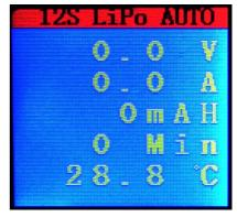
On Auto interface, press Knob for 3 seconds alternate to Idle mode.
