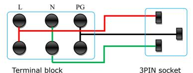
So when connect block to AC source, please note L, N and PG wire must be connected in parallel on AC source.
