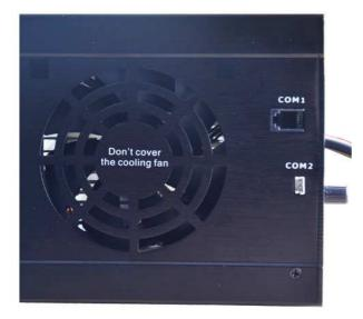
**COM1:** connect to Chargery BMS, the charge current will be controlled by BMS when any cell voltage reach OVP.
